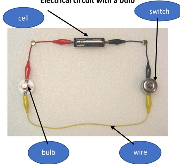
The switch opens and closes the circuit. The bulb lights in this circuit because the switch is on.
